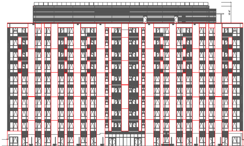
Figure PC2: Precast Panel Typical Layout
